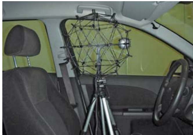
GFal Tech's Acoustic Camera spherical array can measure in-vehicle noise.
