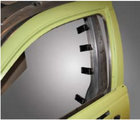
WISEgap sensors from Inora Technologies measure door-seal margins.
